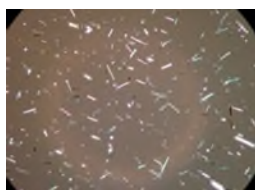
2b) bad solution state caused by non-dissolved fibrous particles
