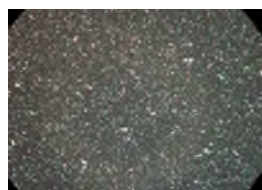
2a) bad solution state caused by solid salt particles
