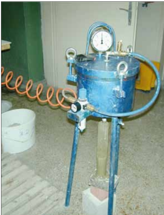
Figure 1. Filter press for testing concrete stability.
