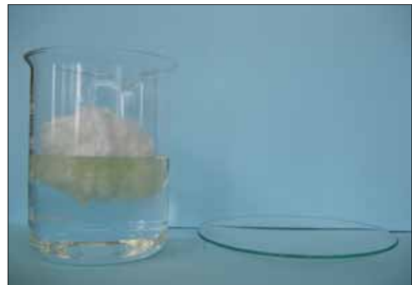
Figure 3. TENCEL®Biosoft floating on water, absorbing peanut oil.
