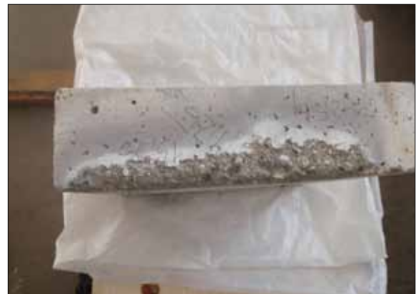
Figure 5a. Spalling of conventional concrete after fire testing.
