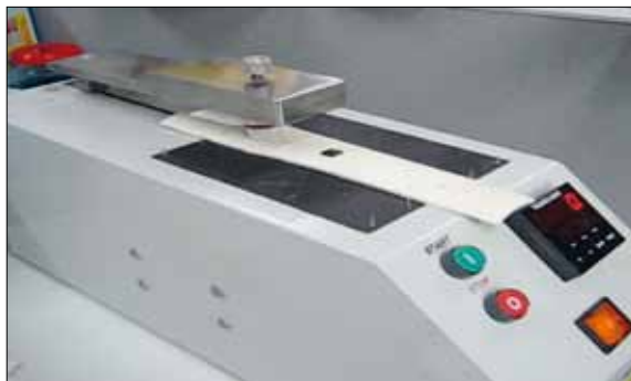
Figure 7. Apparatus to wipe Mascara from artificial skin.
