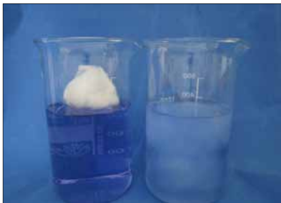
Figure 6. Olea fibres swimming on water compared to standard viscose.
