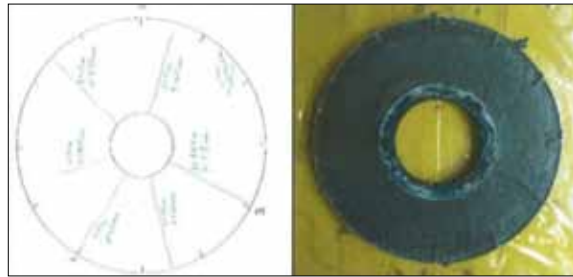
Figure 2. Shrinkage of concrete; left side: crack formation; right side: test apparatus.
