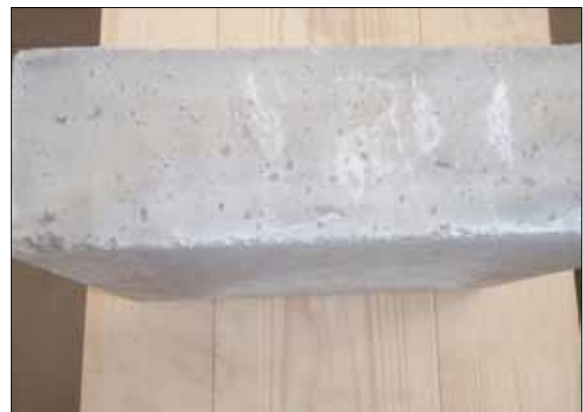
Figure 5b. No spalling of concrete with TENCEL ® after fire test.
