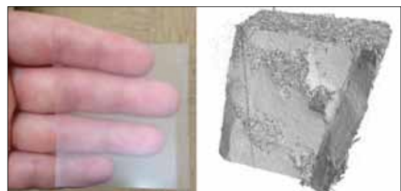
Figure 7. TENCEL® gel coatings on PES foil (left) and pulp paper (right, CT image, 1µm voxelsize).
