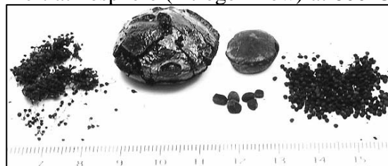
Figure 4. Different carbon aerogels - precursors (left to right): cross-linked, cellulose-acetate, cellulose-carbamate, NaOH/cellulose and NMMO/cellulose.
