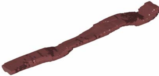
Figure 7. 3D visualization of a detected individual fiber in a kraft paper sample.
